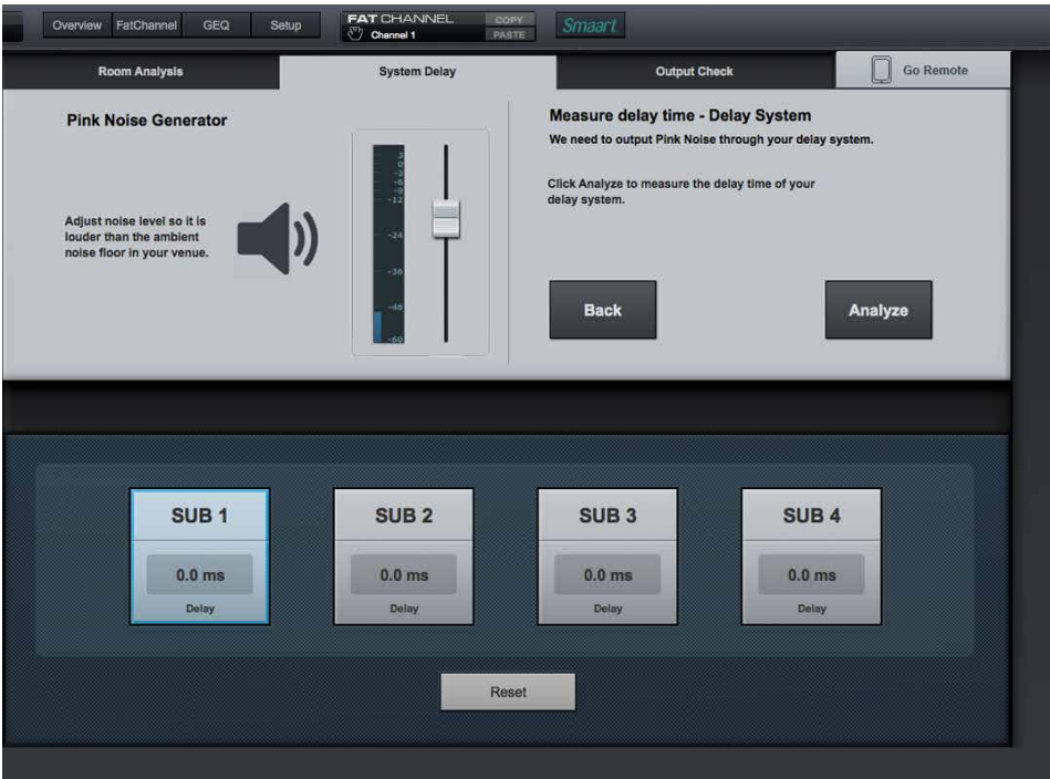
When used with our PRM1 Measurement Microphone, the Smaart Delay Wizard automatically sets the correct delay time — a task that used to require an experienced, professional sound engineer.
