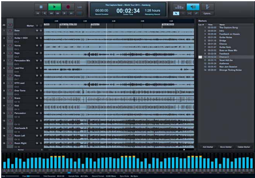
Above: One-click recording: Capture 2.0 for Windows and Mac — free with StudioLive mixers. Below: Capture “maps” the channels on your StudioLive mixer to Capture tracks.
